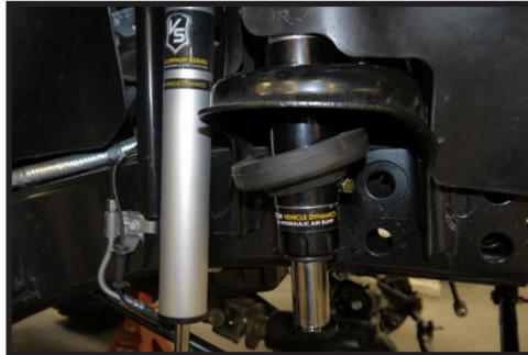
**9.** Reinstall the spring and slowly jack the axle up until you can reconnect the shock, swaybar links, brake line brackets and wiring.
