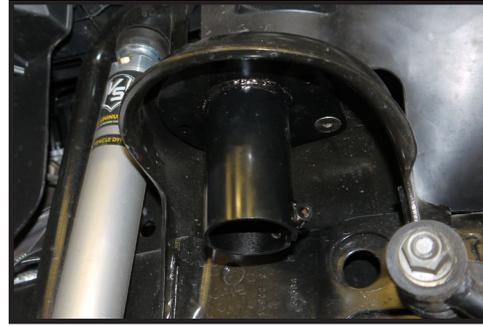
**8.** Slide the factory rubber coil isolator over the bumpstop mount. Preassemble the 1/4" bolt and nut through the pinch tubes. Slide the hydraulic bumpstop up into the mount and tighten the pinch bolt. Do not over tighten. Repeat on opposite side. (FIG.5)
