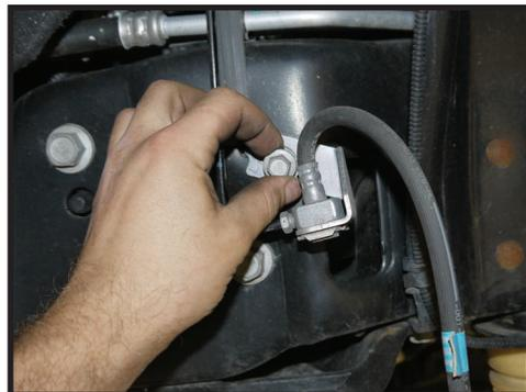
4. On the driver side of the track bar, remove the nut and the upper track bar bolt using (2) 30mm socket/wrenches. [FIGURE 4]
