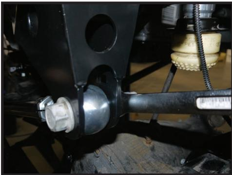
**18.** Remove the steering stabilizer from the factory frame bracket using a 15mm socket/wrench. Remove the bracket from the frame using an 18mm socket/wrench. Remove the steering stabilizer from the drag link using an 18mm socket/wrench, then use a ball joint separator fork or a hammer to break the taper loose and remove the stabilizer.
