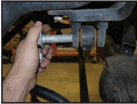
5. Support the axle housing with a jack and remove the front shocks. The shocks are limiting suspension droop so make sure that the axle is well supported or it will fall when the shocks are removed. Use an 18mm socket/wrench to remove the lower bolt, and a 16mm socket/wrench on the stem.
