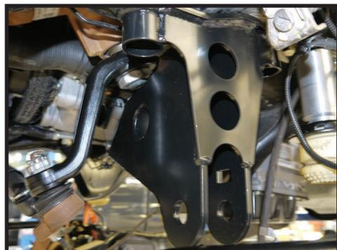
15. Install the new track bar bracket using stock hardware. Hold the track bar bracket in position and insert the stud plate through the crossmember and bracket. Use a small amount of thread locker on threads, and install nuts using a 21mm socket/wrench. Use thread lock on frame bolts and tighten using an 18mm socket/wrench. [Torque to factory spec] [FIGURE 7]
