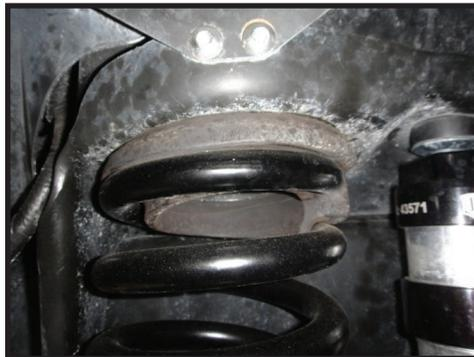
**9.** Slowly raise the axle just before the springs start to compress. Make sure the springs are properly seated before compressing them.
