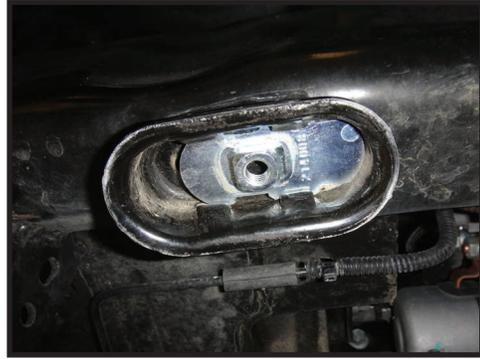
**14.** Mount the bumpstop spacer (217124) to the frame threading it into the retainer plate using the supplied 3/8" hardware, tighten using a 9/16" socket/wrench. [Torque to 30 ft-lbs] Lightly grease and press the bumpstop into the pocket. [FIGURE 8 AND 9]
