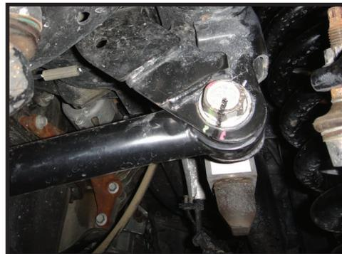
3. Remove the upper track bar bolt from the frame using a 27mm socket/wrench. Use caution as the truck may shift when the bolt is removed. [FIGURE 2]
