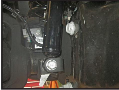
**6.** Slowly lower the jack until the coil springs become loose enough to slide out. Be careful not to damage any brake lines, ABS wires or differential locker wires (Power Wagon only).
