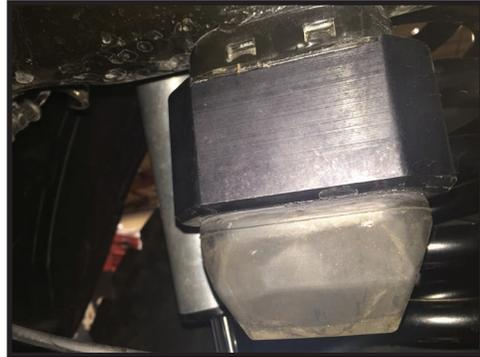
**15.** Connect the sway bar to the stock sway bar links using an 8mm and 18mm socket/wrench. [Torque to factory spec]
