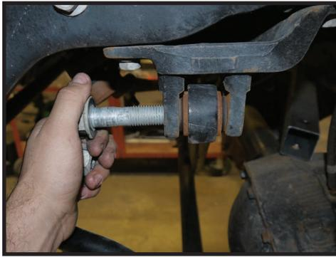
**5.** Support the axle with a floor jack and remove the front shocks. The shocks are limiting droop so make sure the axle is securely supported or it will drop when the shocks are removed. Use an 18mm socket/wrench to remove the lower bolt.
