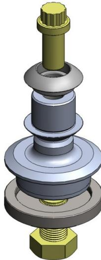
**8.** Install the arm on the ball joint adapter. Fit the uniball dome, make sure that the upper and lower radius meets the curve of the ball, or damage to the uniball may occur. Install the 12pt bolt with the supplied RED thread locker. [Torque to 90 ft-lbs]
